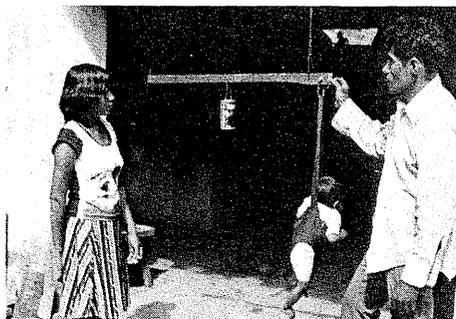
Ideas for several types of homemade scales are given on the next page. Be sure to check the accuracy of your scales from time to time, using objects of known weight.
