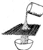
4. Wash some fine sand to remove the dirt. Dry it in the sun, and sift it through a very fine strainer. Then heat the sand to remove moisture.
