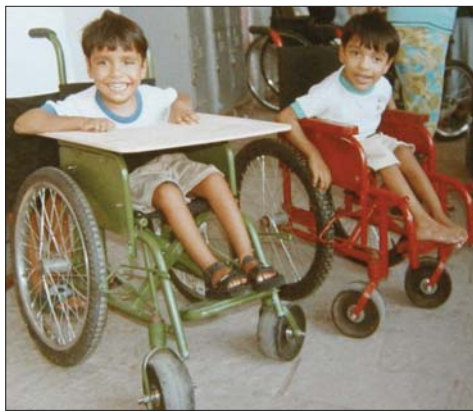
These wheelchairs have broad front tires to assist traveling over rough terrain.
