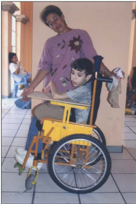
This child with floppy cerebral palsy has low muscle tone and slumps forward when he sits. The adjust-able table on a wheelchair designed at PROJIMO can be raised to lift his arms and shoulders enough so that he can hold up his head. As he gains strength, his mother can lower the table bit by bit.
