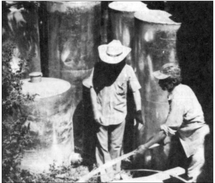
A deaf craftsman in Ajoja helps one of the health workers make sheet metal storage bins for the cooperative corn bank.
