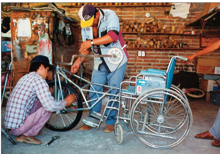
Marcelo was exceptionally creative. Here he develops and builds a removable hand-powered tricycle attachment to a wheelchair for traversing rough terrain more quickly and easily.
